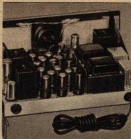
Power stages on separate chassis are removable for flexibility and easy servicing.
