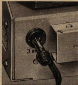
Screw-in type fuse. No tools are needed—you can check or change the fuse in a second.
