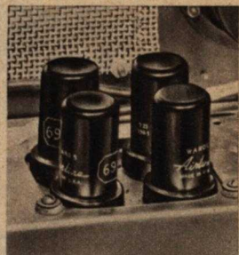
Input tubes rubber mounted on separate chassis eliminate vibration, for quiet operation.
