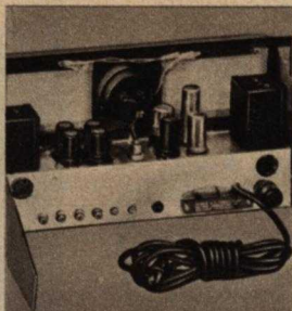
All connections made on terminal strip. Output impedances for any speaker network.
